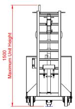
Please see the above general arrangement drawings of the short counterbalance depalletiser (DTP08-250kg) suitable for confined areas. A longer DTP08-350kg with 350kg SWL is available, dimensions are shown below.
